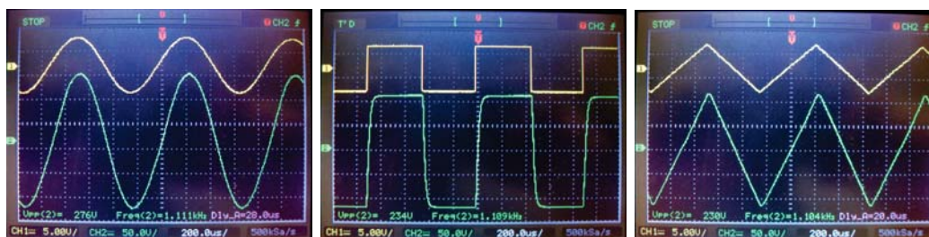
Figure 4: Output response to different waveforms at ~1109 Hz. Yellow - input, green - output.
