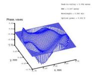
Optical figure of OKO 19-ch piezoelectric DM after active flattening using FrontSurfer wavefront control system. P-V aberration does not exceed lambda/40, while RMS aberration is as good as lambda/100 for lambda=540nm.
