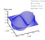
Optical figure of OKO 19-ch piezoelectric DM after coma with amplitude 1.78 waves (lambda=540nm) was formed on the mirror surface.
