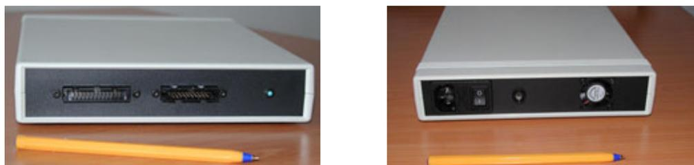
Figure 4: Front and back panels of 20 channel high-voltage amplifier unit.
