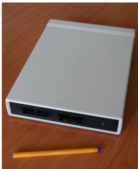
Figure 3: 20 channel high-voltage amplifier unit.
