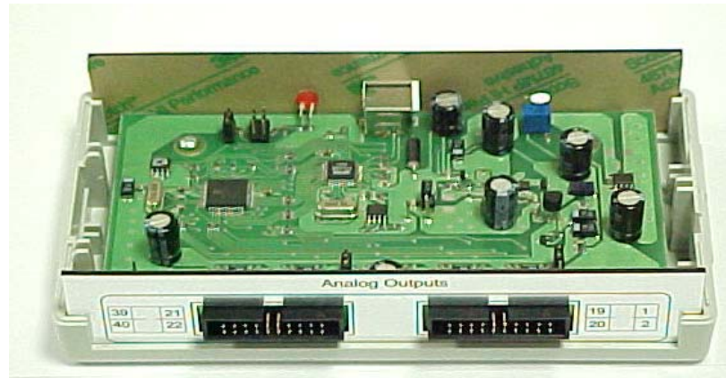
Fig. 1. «DAC-40-USB» view from the output connectors' side
