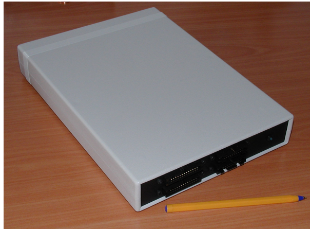
Figure 4: 40 channel high-voltage amplifier unit.
