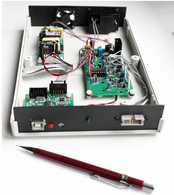
Figure 3: Three-channel high voltage driver includes power supply, USB DAC4, and A4MEMS
