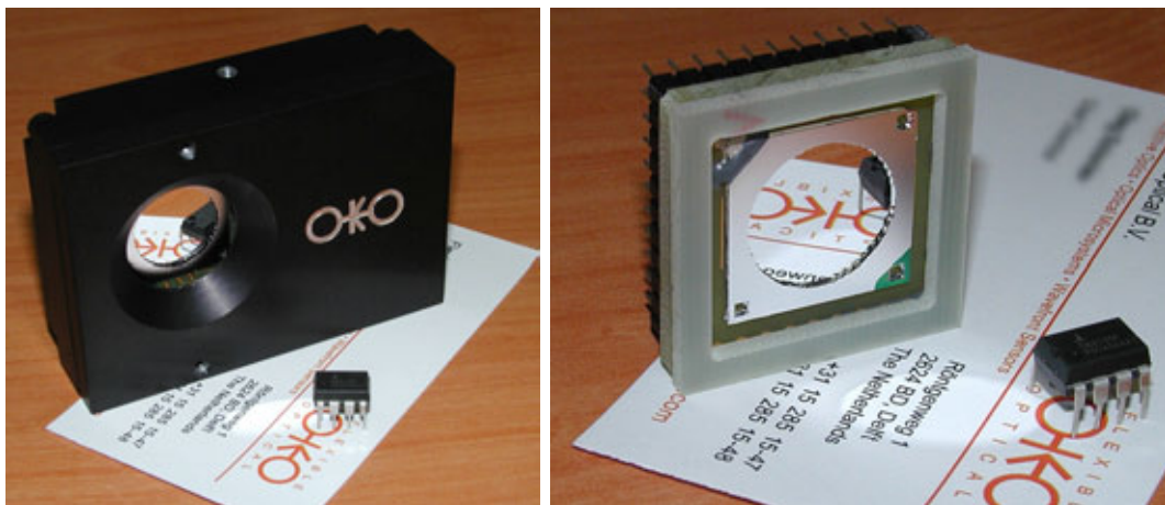
Figure 1: Typical view of a 37-channel micromachined deformable mirror with and without package. Please note that these mirrors can be fabricated with different package designs, so the mirror you have may look differently.
