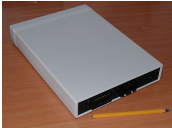
Figure 4: 40 channel high-voltage amplifier unit.
